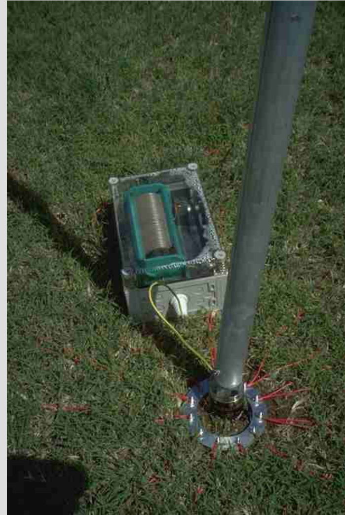
9Y4NW: 80/160m vertical; feedpoint insulator is a rum bottle
