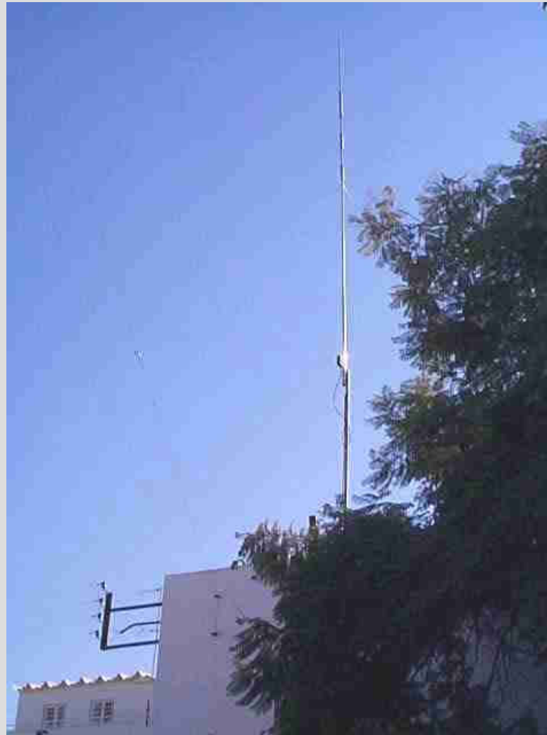
CN8WW: R7000 mounted at CN8MC station
